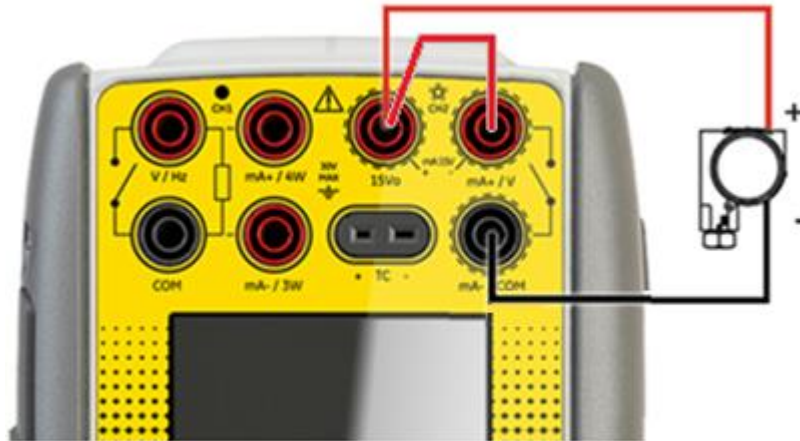
Figure 4-1 Connection with Internal Loop Supply, Parallel HART Connection
