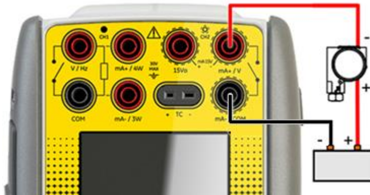
Figure 2-1 Connection with External Loop Supply
